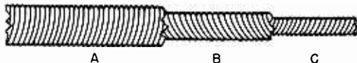
FIG. 1. Typical construction of remote control shaft. Note three layers, A, B, and C, which are made up of spring-steel wire, wound in opposite directions for stiffness and to eliminate backlash.
